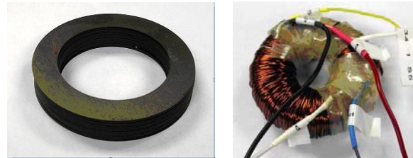
Fig. 1. Appearance of measured steel lamination ring core and coils
